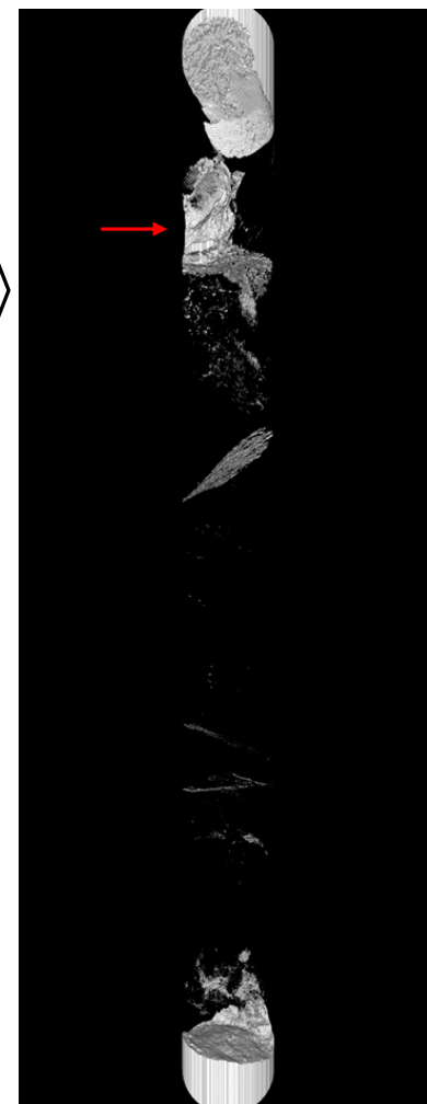
Cracks and pores
