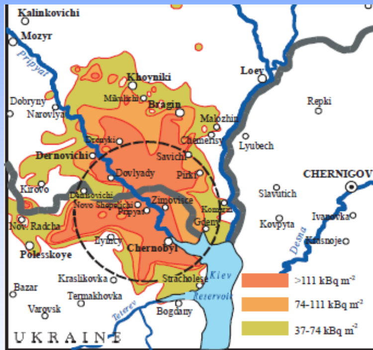
FIG. 3.8. Surface ground deposition of ^{90}\text{Sr} [3.4].
