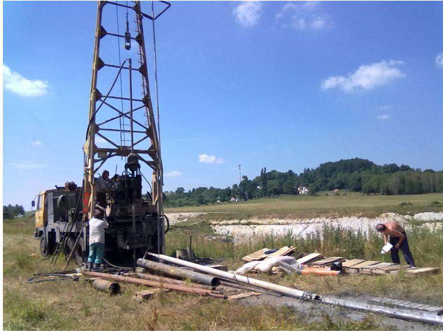
**Fig. 3.1** Truck-mounted drilling rig (ZIF-650M) in operation at the Ruprechtov site
