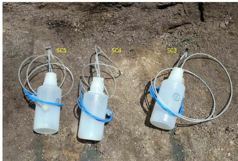
**Fig. 3.4** Soil water sampling using suction-cups - figure shows sampling bottles above-ground; the suction cups themselves were installed at various depths (app. 30 – 90 cm)
