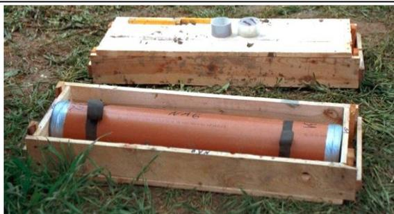
*Air-tight sealed drill core for transport and storage of redox-sensitive material*
