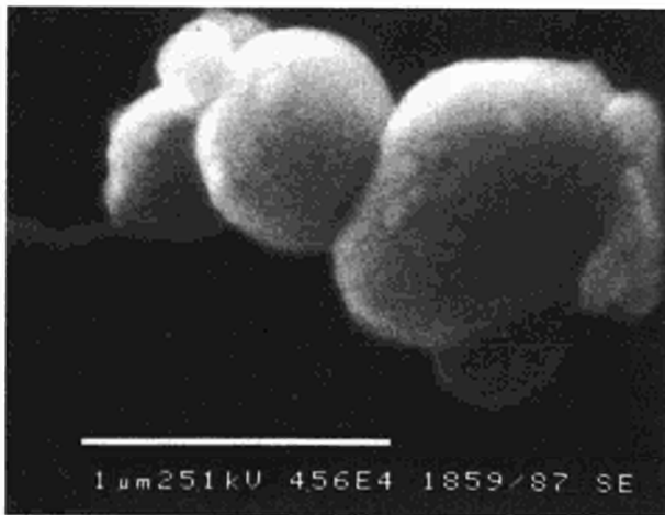
Figure Vb. Cross-flow ultrafilter prepared from aqueous colloid concentrate (EIR): Typical field of view showing colloid aggregate.
