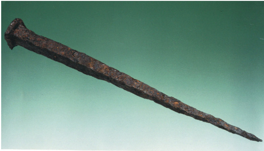
Figure 2 A photograph of one of the nails (c.35 cm long) from the central part of the hoard at Inchtuthil. There is an excellent state of preservation despite over 1860 years of burial (from Miller et al., 2000).
