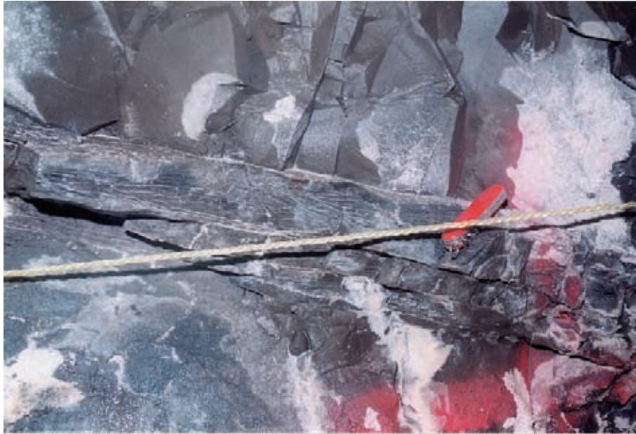
Figure 2-9a. Typical infilled fractures at sampling site M2, Adit A-6. Several main fractures, 2–10 cm apart, with fine anastomosing network of veinlets between them (from Alexander and Mazurek, 1996).
